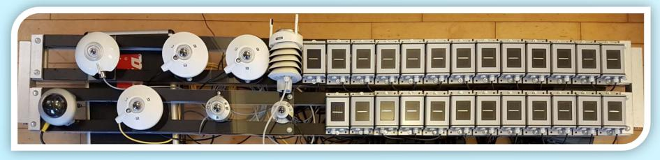
Calibration rig with weather station
