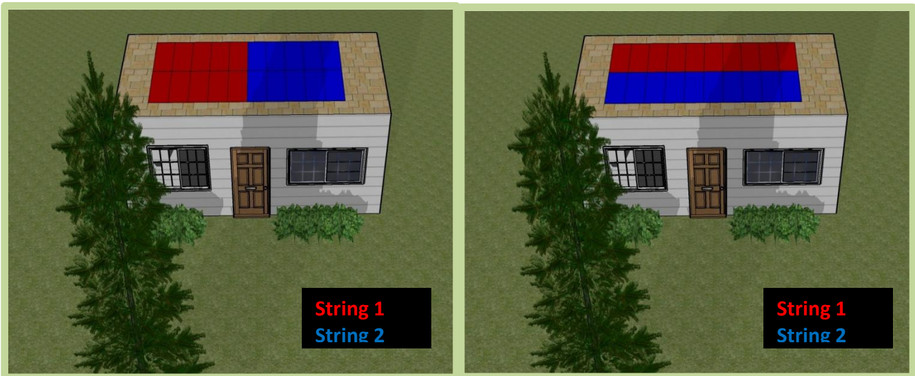
Isolated Shading – One string in array is shaded
