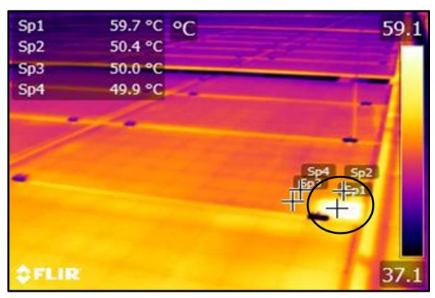
Figure 37: Modules with uneven stains on glass were seen to have developed hotspots with  $\Delta T \sim 10^{\circ}$ C.
