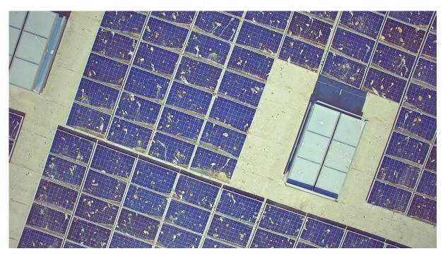
Figure 8: Aerial view of a rooftop commercial PV plant installed at a coastal site, presenting severe issues of localized soiling due to dirt (bird droppings) © CEA-INES.
