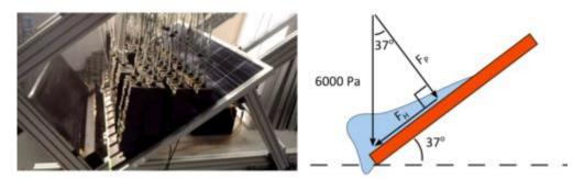
Figure 54: Left) IML test setup [169] using even weights on a pitched module installation. Right) A simplified force diagram that simulates the effects of settled snow.
