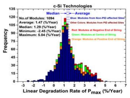
Figure 29 DEGRADATION RATE Histogram of linear degradation rates of  $P_{\text{max}}$ : All c-Si PV modules in which modules from PID affected sites differentiated along with their position in the string.
