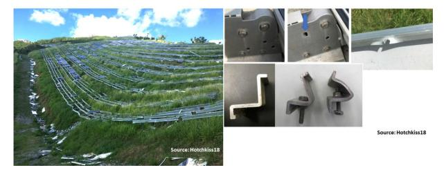
Figure 43: Damages of PV facilities by hurricanes in U.S. Virgin Islands in 2017.
