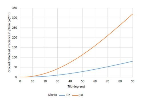
Figure 46: Ground reflected irradiance calculated as function of module tilt angle and different albedo at horizontal irradiance of 800 W/m<sup>2</sup>, using Eq. (17).
