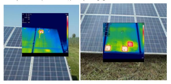
Figure 14: Impact of bird droppings and locally increased temperature (left), Impact of freshly cut green and unexpected hotspots (right) [Fraunhofer ISE].
