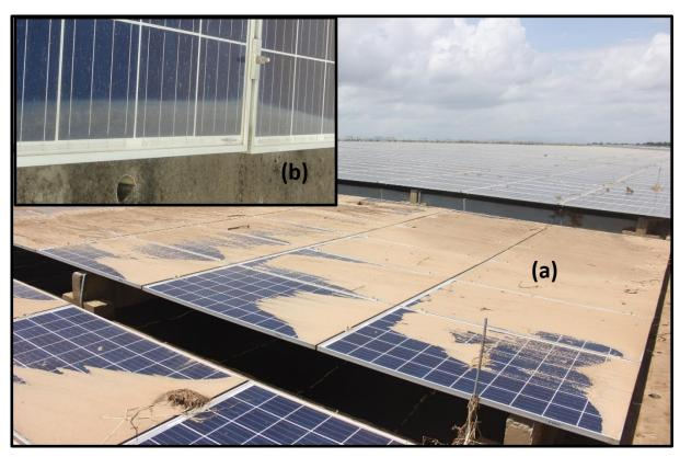
Figure 36: (a) Silt was seen to be deposited post-flooding on most of the low inclination angle mounted modules in P2. (b) Uneven stains were observed near the bottom edge of most of the modules which could not be removed even after cleaning with soap water and scrubbing.
