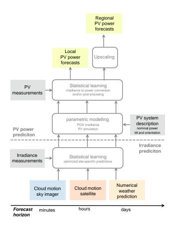
Figure 5: Overview of basic modelling steps in PV power prediction. Adapted from [49].
