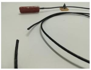
Figure 12: Cable bitten by a marten (left) (pveurope.eu © Leitl). Temperature sensor cable cut in half by a rodent (right) [Eurac Research].
