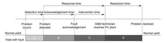
Figure 2: Timeline from fault to resolution, showing the O&M KPIs related to response and resolution time, and the associated yield losses for each phase. In many cases, the detection time will be very short, although this depends on the nature of the SCADA system and the type of fault. Depending on the contractual framework, the yield loss
