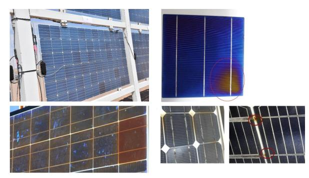
Figure 25: Degradation mechanisms evidenced in PV power plants installed in the Atacama Desert.
