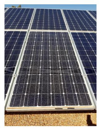
Figure 21: PV module damaged during vegetation management due to pebbles. Array in Central Australia.
