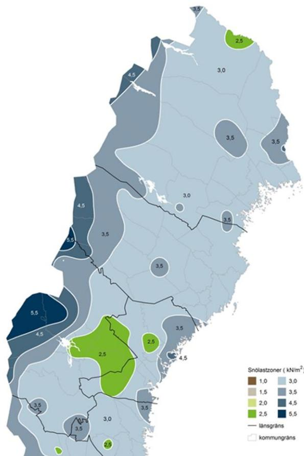
**Figure 56: Snow load zones north of 60°N in Sweden, where it is most important to consider snow loads when constructing a building. The numbers given in this map range between 2.5 kN/m<sup>2</sup> and 5.5 kN/m<sup>2</sup>. They can be used to dimension for extra roof loads due to snow when constructing a building in the regions described in the Swedish application of Eurocode 1 [171].**
