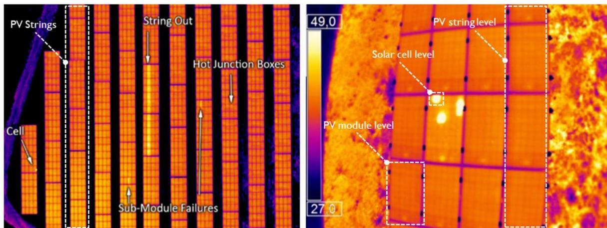
Figure 9: Aerial IR imaging by aircraft (left) and drone (right), revealing different failure modes at cell, submodule, module, and string level © Heliolytics Inc. (left image), © CEA-INES (right image).
