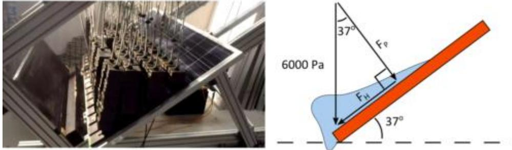
**Figure 54: Left) IML test setup [169] using even weights on a pitched module installation. Right) A simplified force diagram that simulates the effects of settled snow.**
