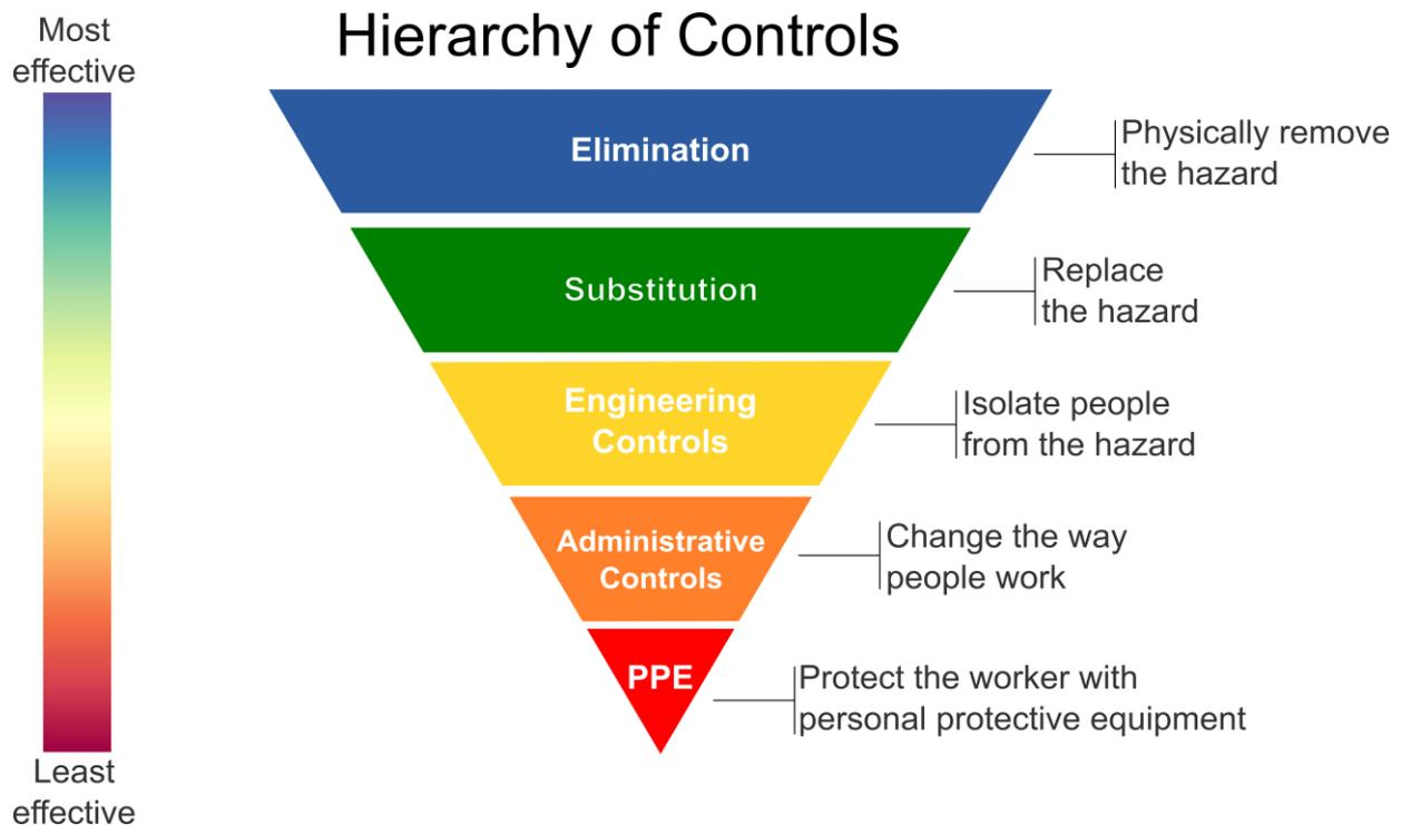
**Figure 6: Hierarchy of controls, adapted from [63].**
