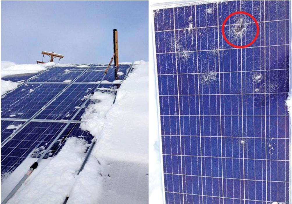
Figure 52: Careless removal of snow may destroy the surface of PV modules [166].
