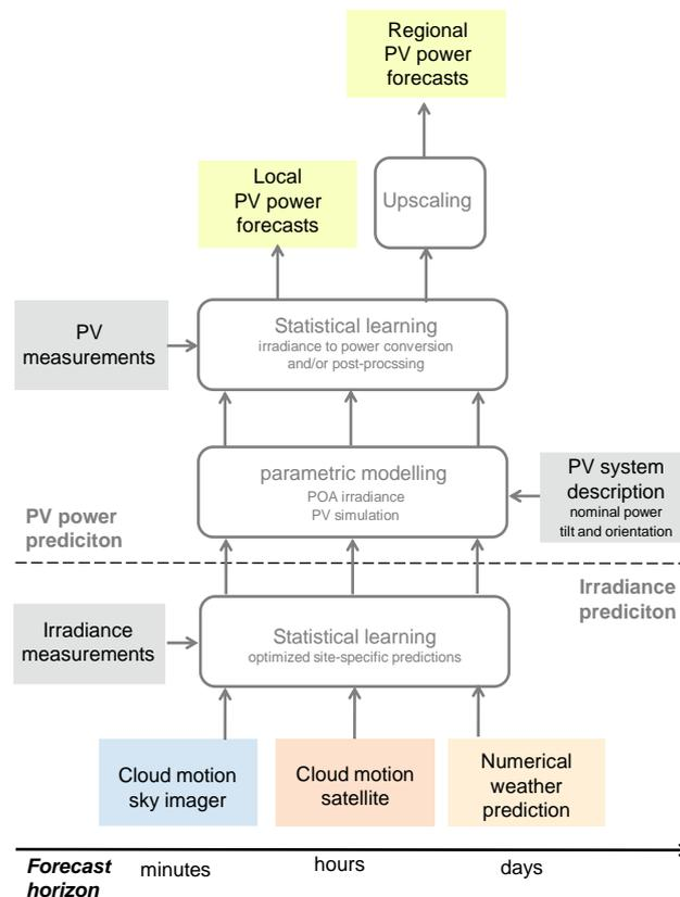
**Figure 5: Overview of basic modelling steps in PV power prediction. Adapted from [49].**
