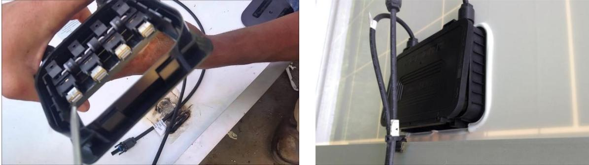
**Figure 27: Failures in a junction box in operation during about a year due to degradation issues.**
