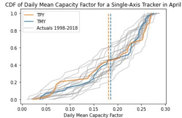
The figure demonstrates the daily averages of capacity factor (CF) (Y-axis) for one location/pixel for the month of April for single axis scenario for TPY and TMY. It is showing that the typical datasets have differences.
