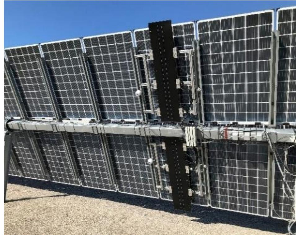
Backside of a  $2P_{\text{Gap}}$  system. The black mini modules contain 10 cSi cells to measure  $R_{\text{POA}}$  nonuniformity
