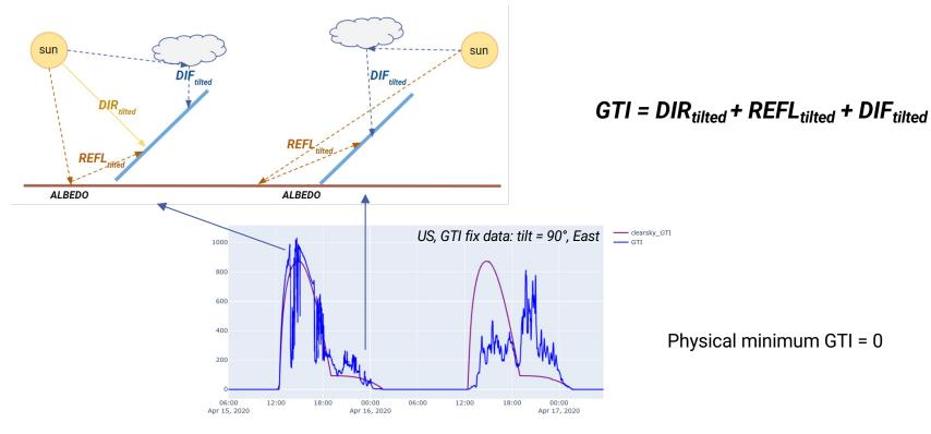
Direct tilted irradiation DIR<sub>tilted</sub> = DNI \* cos(incidence\_angle)
