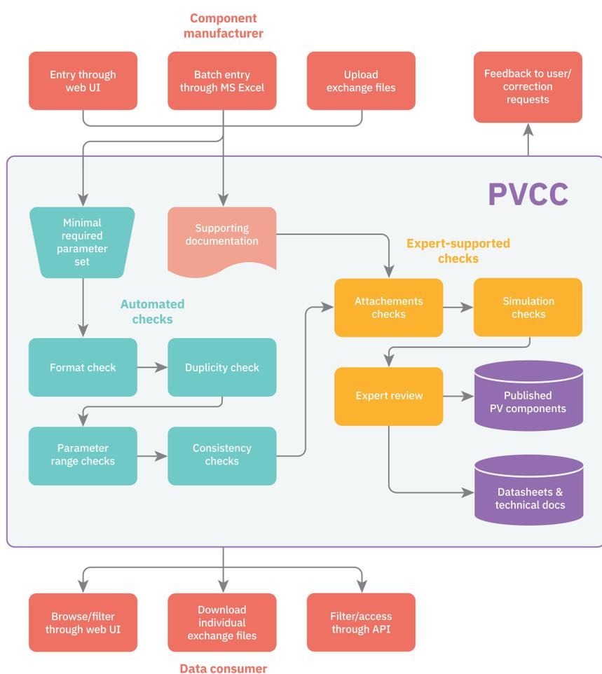
Figure 1: Schematic representation of the PVCC, its input and output options, and the parameter verification and validation chain.
