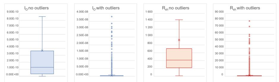
Figure 2: Spread of values of the reverse diode saturation current ( $I_0$ ) and shunt resistance ( $R_{sh}$ ) parameters in the California Energy Commission database of PV modules [1].
