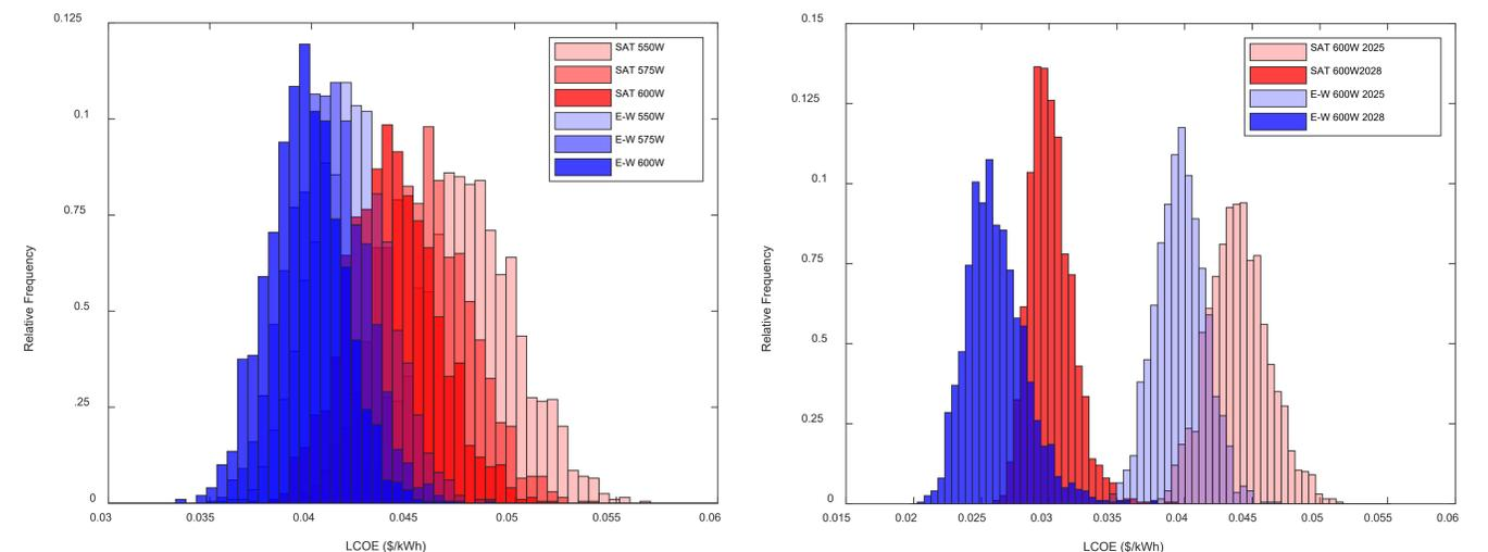
Figure 3: A) LCOE histogram for SAT and E-W systems in 2025 with 550, 575 and 600 W modules. B) LCOE histogram for SAT and E-W systems with 600 W modules in 2025 and 2028.
