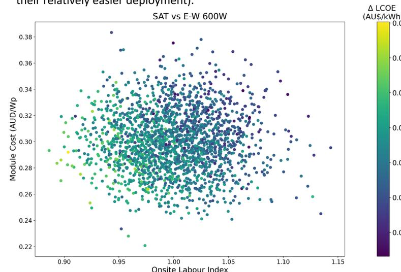
Figure 4: 2-D scatter plot of  $\Delta$ LCOE for an E-W system compared to a SAT system using 600 W modules.
