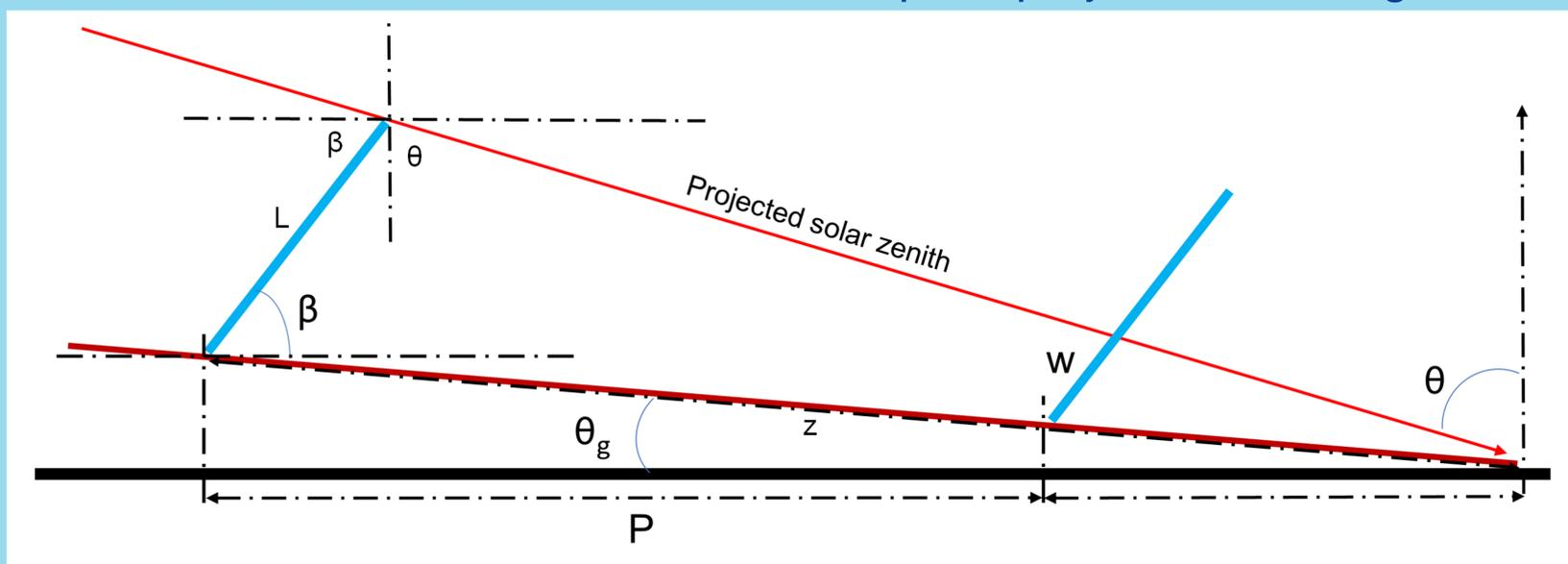
Figure 2: shows the generic case for trackers at any position on sloping terrain.
