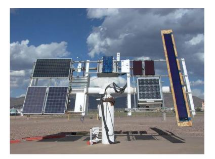
Outdoor characterization is performed on a flexible, fully programmable two-axis solar tracker.
