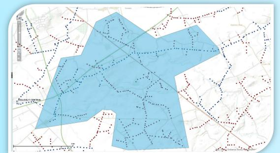
11kV rural feeder measurement area and network topology
