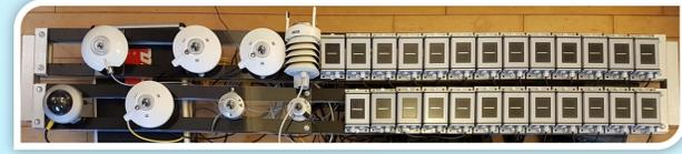
Calibration rig with weather station
