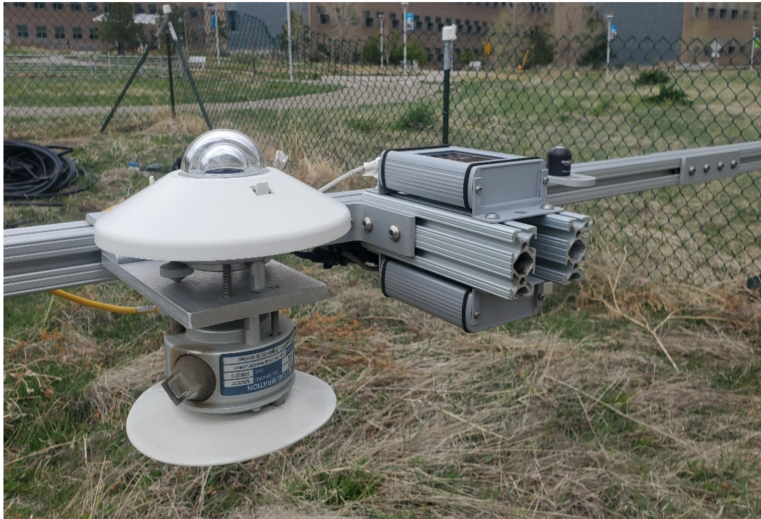
Figure 23 – Experimental albedo measurement test stand with three different types of albedo sensors (Photo credit: NREL).
