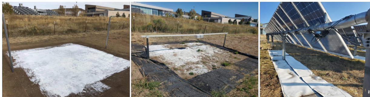
Figure 14 – (left and center) - Commercial solution of spray coating albedo enhancer, 2 years on field [50]. (right) Soiling visible on a plastic-like material albedo enhancer. Photo Credits: NREL (left), Silvana Ovaitt (center-right).
