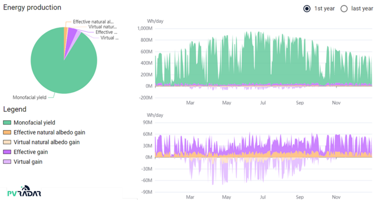
Figure 12 – Screenshot from PVRADAR software showing the effective and virtual bifacial gain (normal ground) and extra gain from optimally applied albedo enhancing materials.
