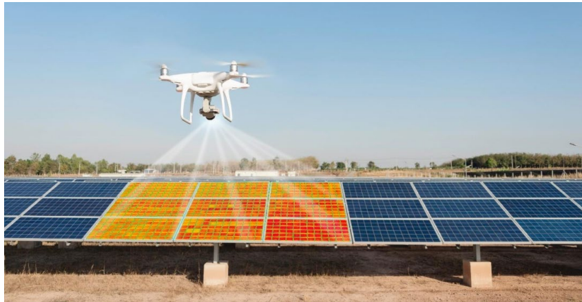
Figure 18: A stylized image showing aerial IR imaging conducted by a drone [79].
