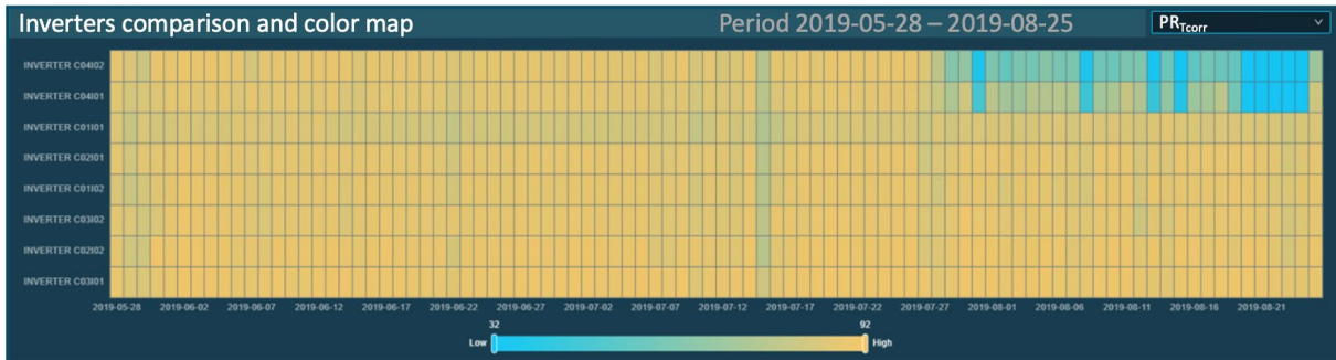
Figure 14: Screenshot of a heatmap representation with PR_{Tcorr} calculations for many inverters in analytics software tools [37].
