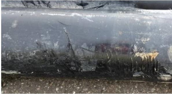
a) Rubbing damage on an HDPE part
