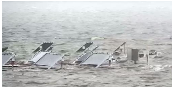
d) Loss of mechanical integrity due to wave forces
