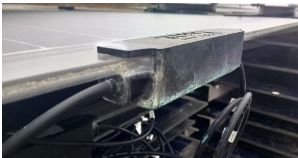
g) Corroded junction box
