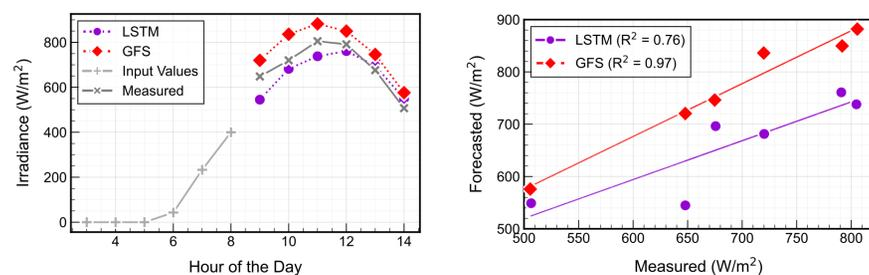
Figure 2. Forecasted solar irradiance (left); Correlation between measured and forecasted irradiance (right).
